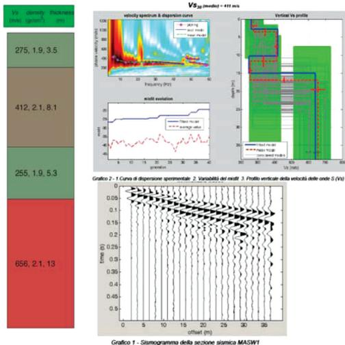
Figure 16. Seismic parameters elaboration derived from MASW test.
