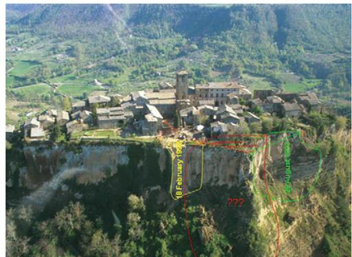
Figure 4. View of the northern side of the cliff and displaying recent phenomena and the of the joints (dotts) isolating an important rock slide (red).
