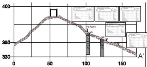
Figure 17. Geotechnical section along the southern side from penetrometric tests and MASW.
