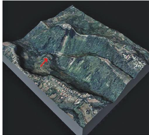
Figure 5. DEM of the area with superimposed an aerial photograph. In the left side it is possible to notice the toe of the large slide that, in 1114 A.D. moved the river from the natural linear behaviour towards the Civita cliff, Northern sector.
