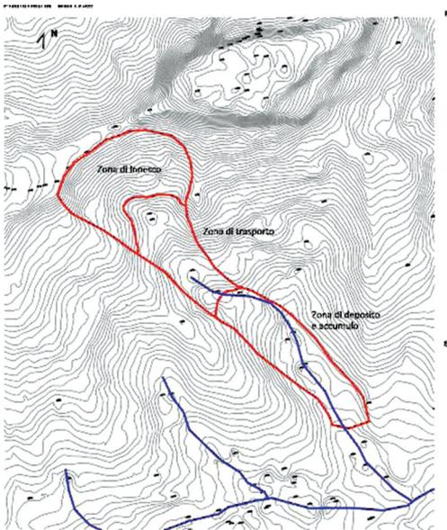
Figure 11. Geomorphological zoning of the southern part of the saddle, in terms of source, transportation and accumulation for triggered earth flow.
