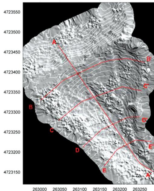
Figure 12. Digital elevation model of the area of the south side with overlapping contours (spacing 5 m) and showing the position of the sections produced.
