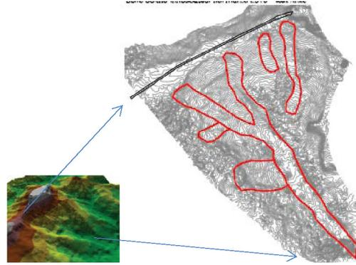
Figure 8. Earth flow instability along the south slope—March 2010.
