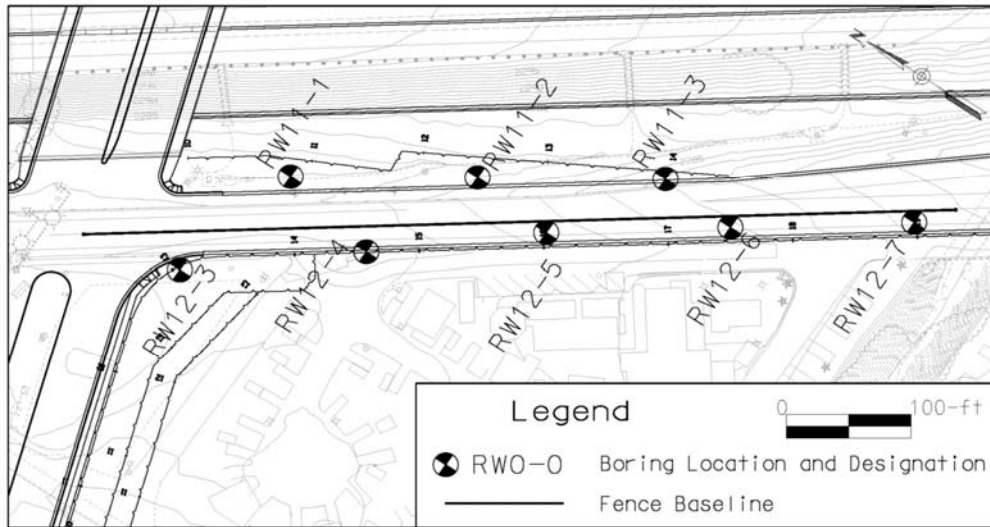
Figure 11-3. Example boring location plan for retaining walls RW-11 and RW-12 retaining an on-ramp to a freeway.
