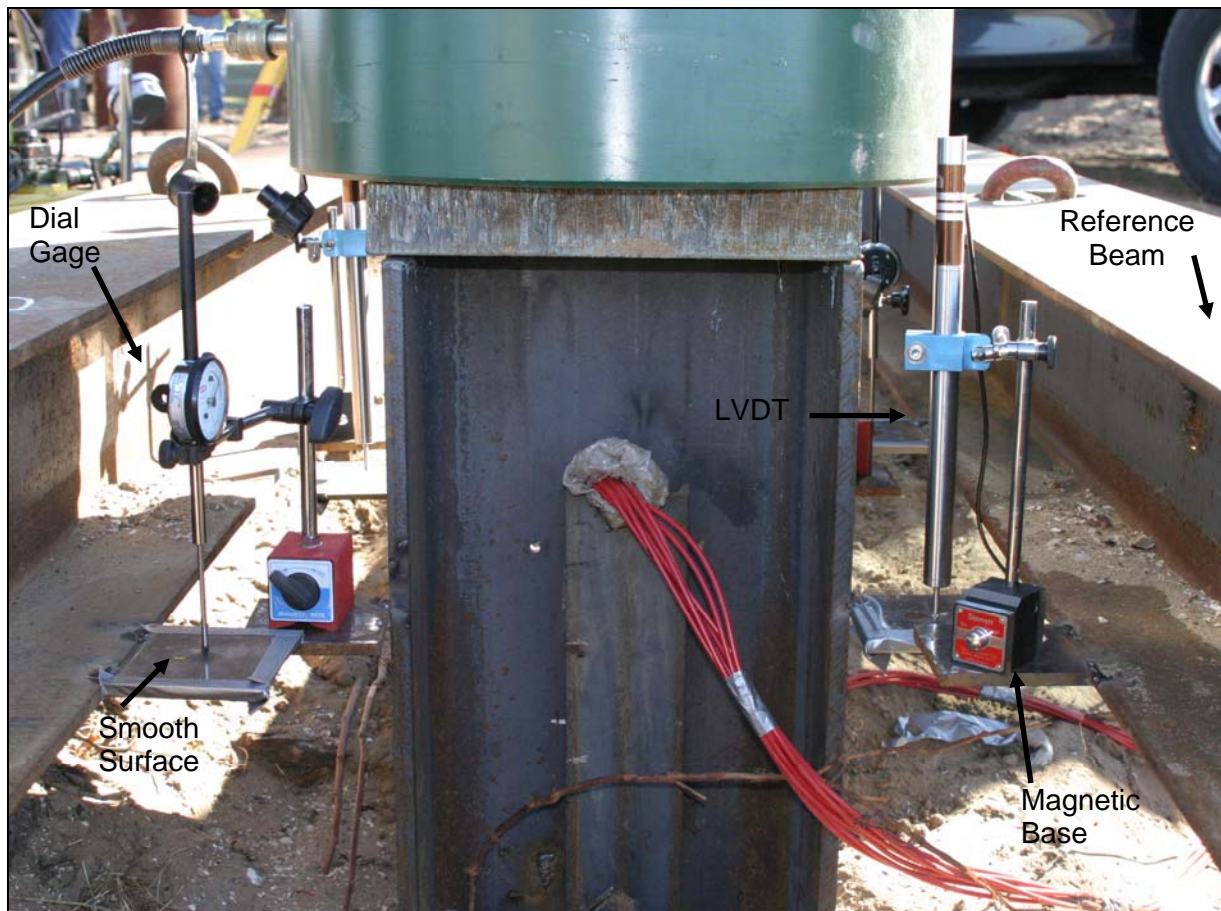
Figure 9-65. Load test movement monitoring components (FHWA, 2006a).
