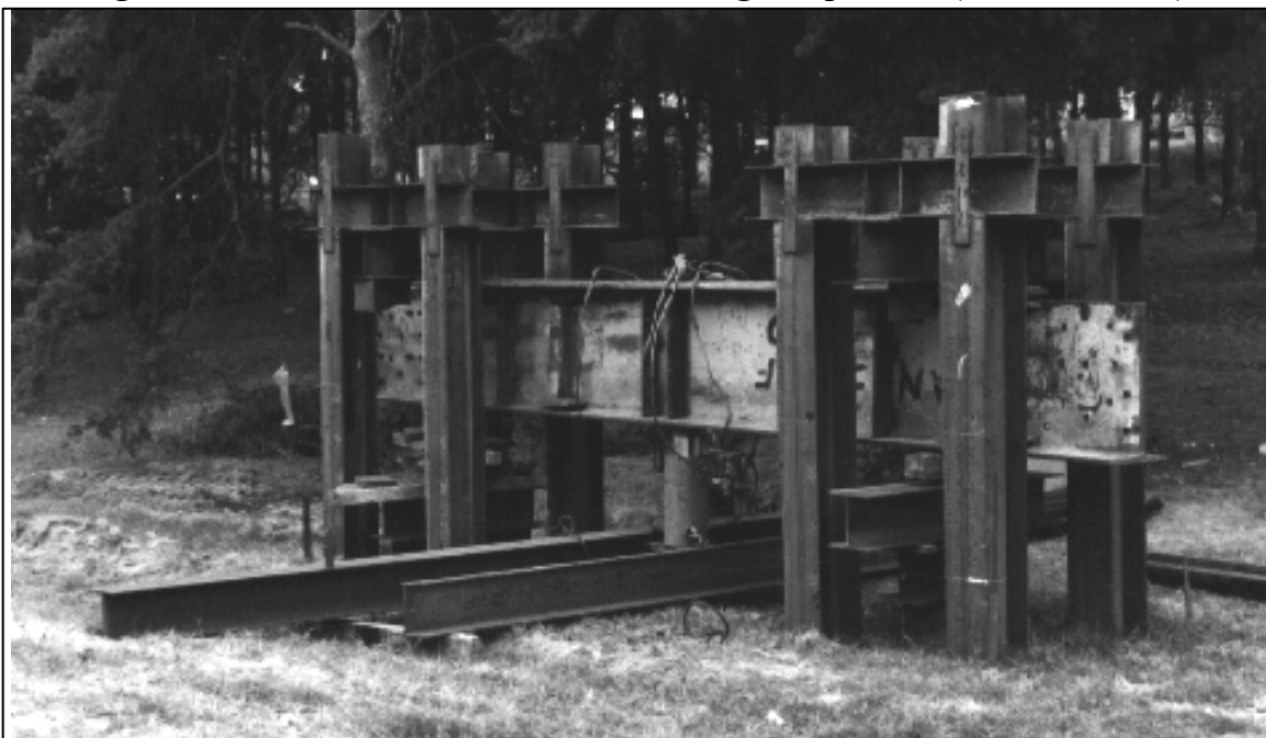
Figure 9-66. Typical compression load test arrangement with reaction piles (FHWA, 2006a).
