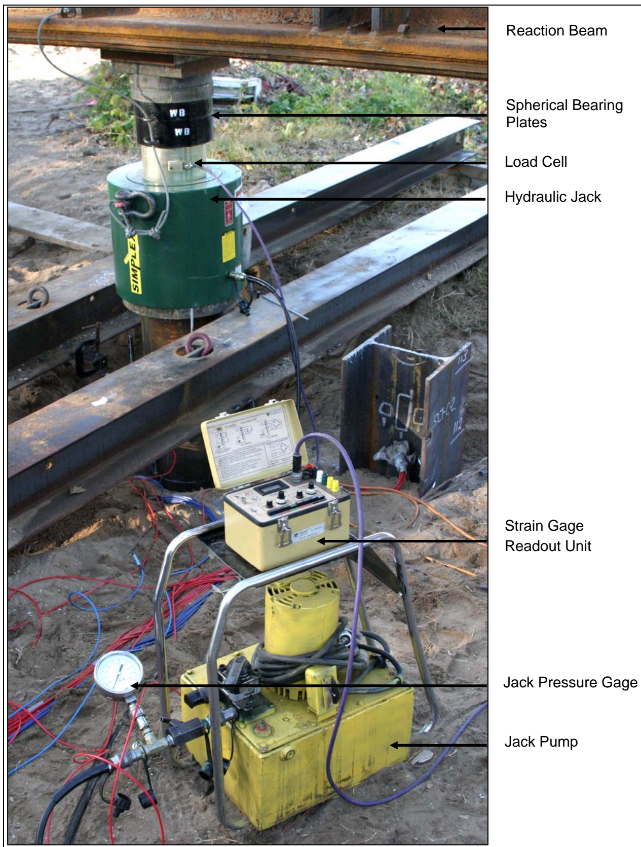
Figure 9-64. Load test load application and monitoring components (FHWA, 2006a).
