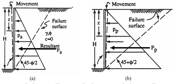
Active pressure at depth z:  $p_a = K_a \gamma z$ Active force within depth z:  $P_a = K_a \gamma z^2/2$
