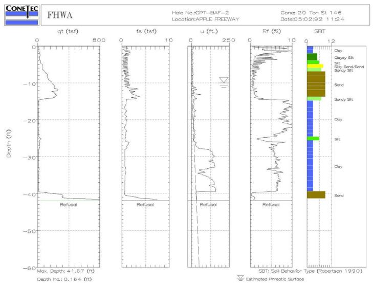
Figure 3-30. Piezo-cone results for Apple Freeway Bridge.
