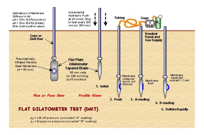
Figure 3-32. Dilatometer test equipment and procedure (FHWA 2002b).
