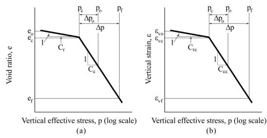
Figure 7-12. Typical consolidation curve for under-consolidated soil – (a) Void ratio versus vertical effective stress and (b) Vertical strain versus vertical effective stress.
