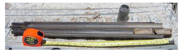
Figure 3-8. Split barrel sampler.
