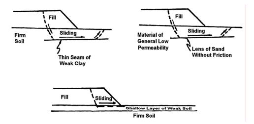
Figure 6-21. Sliding block failure mechanism.
