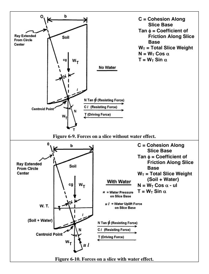
$W_T = \gamma_t \times \text{Average Slice Height} \times \text{Slice Width}$  6-17
