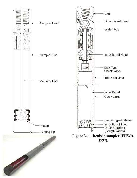
Figure 3-10. Stationary piston sampler schematic (after ASTM D 4700) and photo (FHWA, 2002b).
