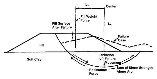
Figure 6-5. Typical circular arc failure mechanism.
