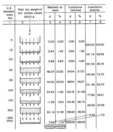
Figure 5-2. Example grain size distribution based on sieve analysis (Jumikis, 1962).
