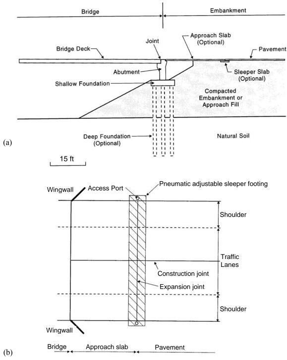
Note: This plan detail is only one way of handling the bridge/fill interface. An approach slab with expansion between the superstructure and the approach slab without a sleeper slab is another.
