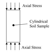
Figure 5-13. Schematic of an unconfined compression test.
