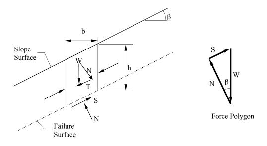
Figure 6-3. Infinite slope failure in dry sand.
