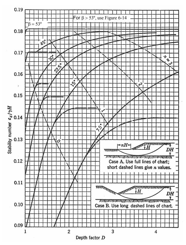
Figure 6-15. Taylor's chart for  $\phi' = 0$  conditions for slope angles ( $\beta$ ) less than 54° (after Taylor, 1948).
