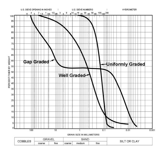
Figure 2-3. Sample grain size distribution curves.
