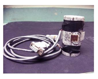
(a) (b) Figure 5-36. (a) Unconfined compression strength test on intact rock core, (b) Use of strain gage on intact rock core sample for measurement of stress-strain characteristics. (Photographs courtesy of Geomechanics Laboratory, University of Arizona).
