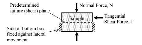
Figure 5-17. Schematic of the Direct Shear Test.
