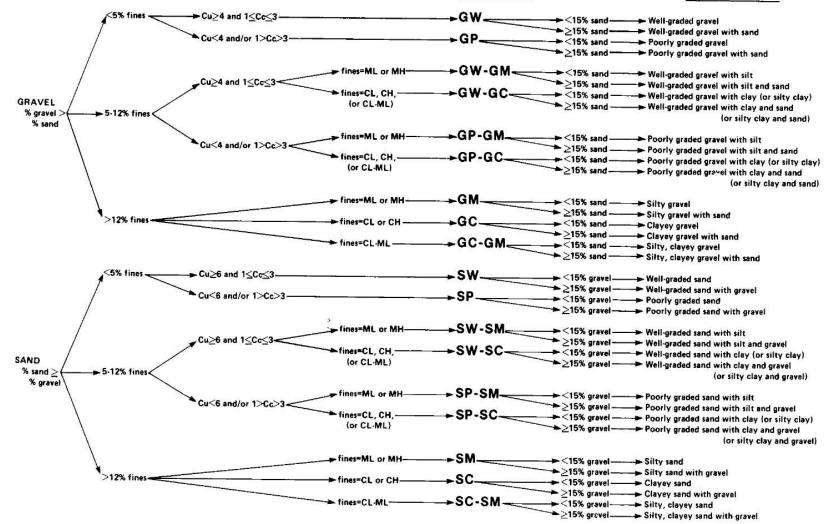
Figure 4-1: Flow chart to determine the group symbol and group name for coarse-grained soils (ASTM D 2487).
