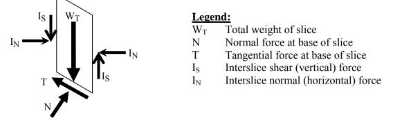
Figure 6-12. Typical static forces on a slice of sliding mass without seepage.
