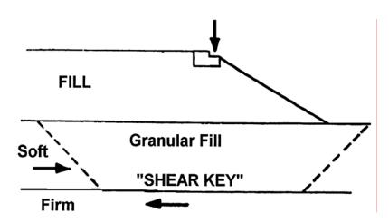
Figure 6-26. Use of shear key to improve slope stability.
