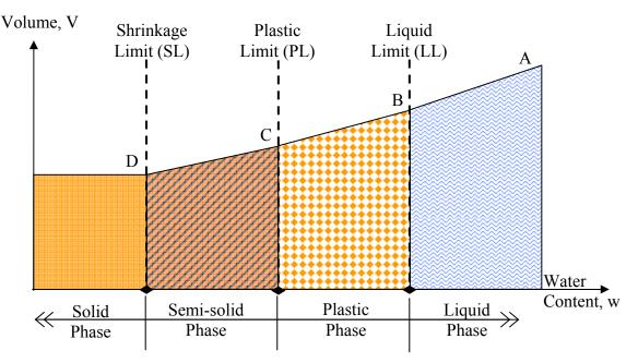
Figure 2-5. Conceptual changes in soil phases as a function of water content.
