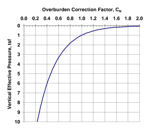
Figure 3-24. Variation of overburden correction factor, C<sub>N</sub>, as a function of vertical effective stress.
