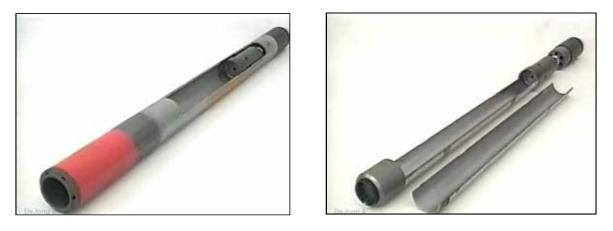
(a) (b) Figure 3-15. Double tube core barrel. (a) Outer barrel assembly (b) Inner barrel assembly (FHWA, 2002b).
