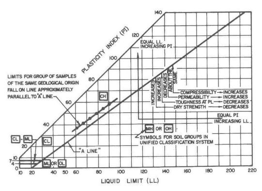
Figure 2-6. Plasticity chart and significance of Atterberg Limits (NAVFAC, 1986a).
