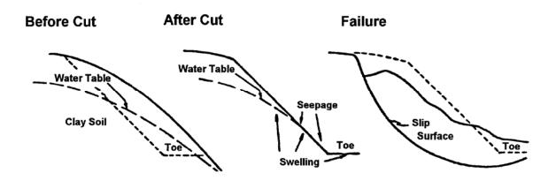
Figure 6-30: Typical cut slope failure mechanism in clay soils.
