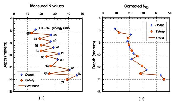
Figure 3-23. SPT N-values from (a) Uncorrected data, and (b) Corrected to 60% efficiency (Data modified after Robertson and Campanella, 1983).
