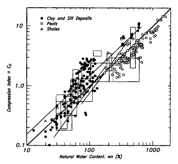
Figure 5-9. Empirical correlation between compression index and natural (in-situ) water content (from Terzaghi, *et al.*, 1996).
