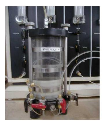
Figure 5-25. Flexible wall permeameter (Photograph courtesy of GeoComp Corporation).
