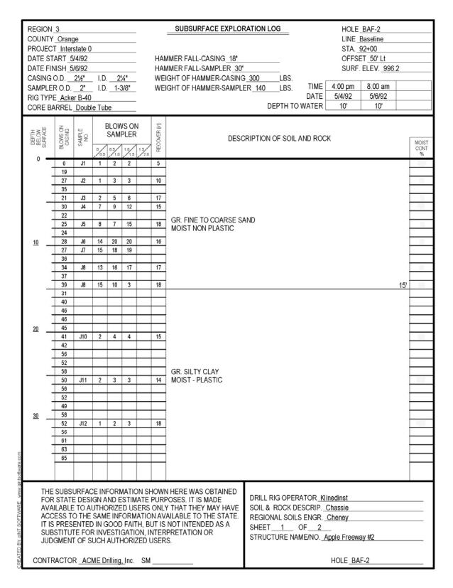
Figure 3-25a. Example subsurface exploration log (0 – 35 ft depth).
