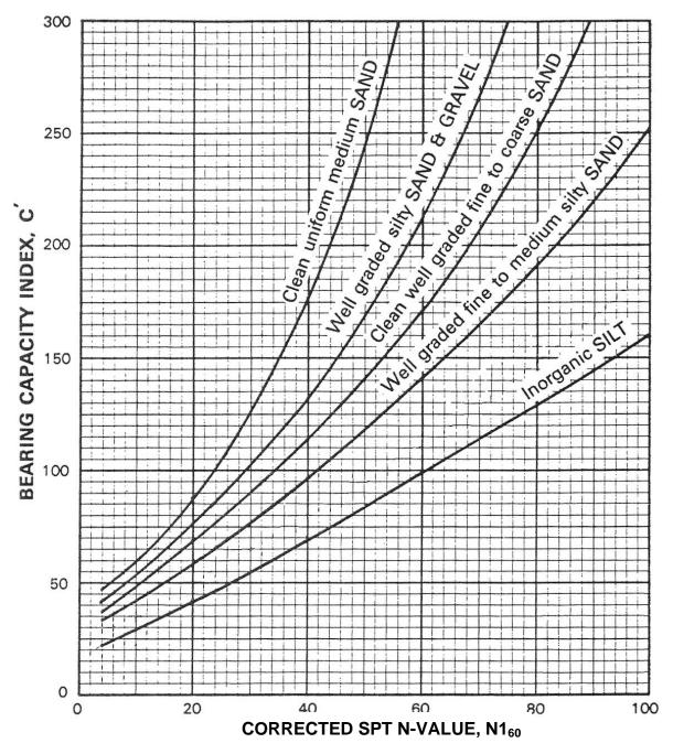
(Note: The "Inorganic SILT" curve should generally not be applied to soils that exhibit plasticity because N-values in such soils are unreliable)
