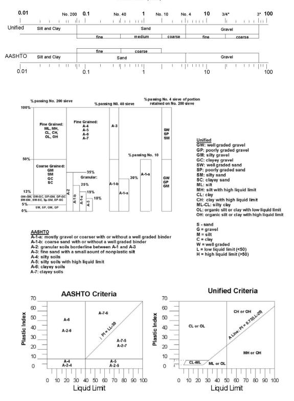
Figure 4-6. Comparison of the USCS with the AASHTO soil classification system (after Utah DOT – Pavement Design and Management Manual, 2005).
