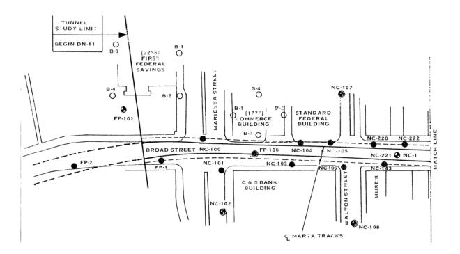
Figure 4-8. Example boring location plan (FHWA, 2002a).
