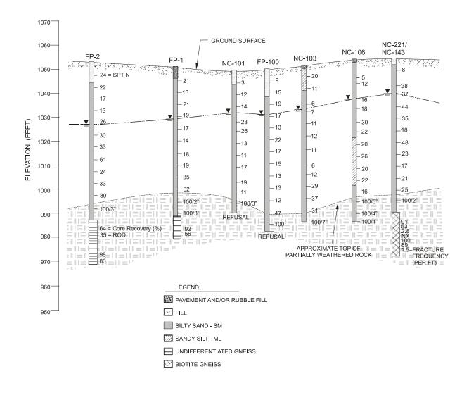
Figure 4-9. Example interpreted subsurface profile (FHWA, 2002a).
