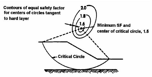
Figure 6-13. Location of critical circle by plotting contours of minimum safety factors for various trial circles.
