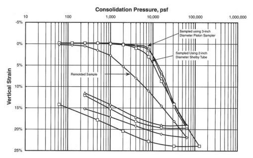
Figure 7-8. Effect of sample disturbance on the shape of the one-dimensional consolidation curve (Reese, *et al.*, 2006).
