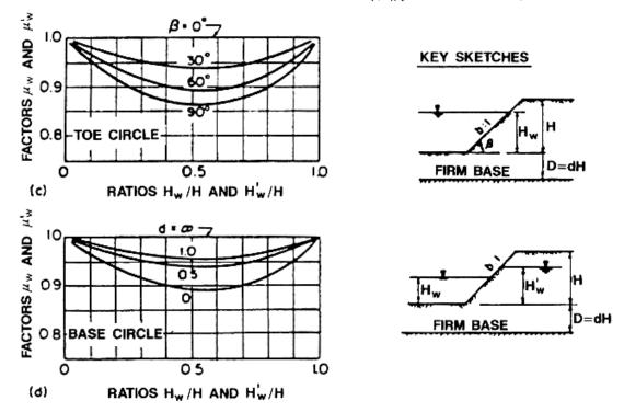
Figure 6-18. Reduction factors to account for surcharge (upper) and submergence and/or seepage (lower) to be used with stability charts for  $\phi=0$  and  $\phi > 0$  soils (Janbu, 1968).
