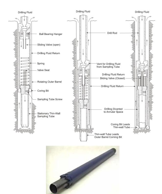
Figure 3-12. Pitcher sampler (FHWA, 1997, 2002b).
