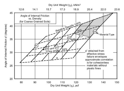
Note: Use caution in the shaded portion of the chart due to the potential for unreliable SPT N-values in gravels
