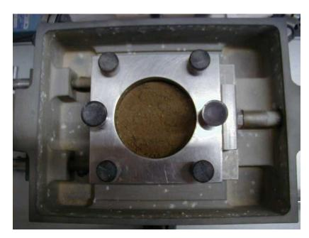
Figure 5-19. Soil sample mounted in direct shear testing apparatus (Photograph courtesy of GeoComp Corporation).
