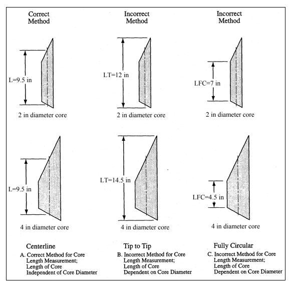
Figure 3-18. Length measurements for core RQD determination (FHWA, 1997).
