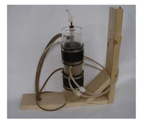
Figure 5-24. Rigid wall permeameter (Photograph courtesy of GeoComp Corporation).
