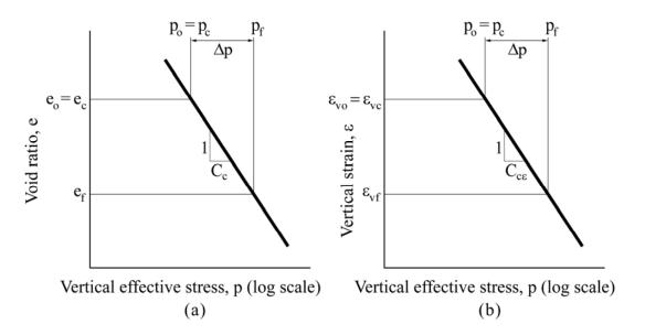
Figure 7-10. Typical consolidation curve for normally consolidated soil, (a) Void ratio versus vertical effective stress and (b) Vertical strain versus vertical effective stress.
