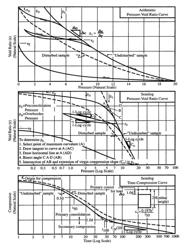
Figure 5–8. Consolidation test relationships (after NAVFAC, 1986a).
