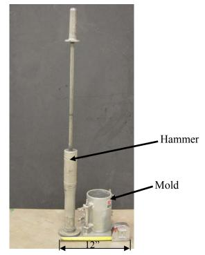
Figure 5-30. Hammer and mold for laboratory compaction test (tape measure is for scale purpose only).
