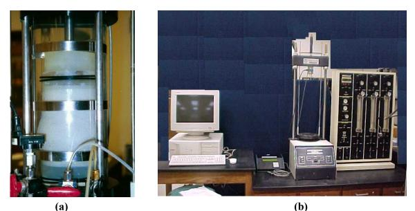
Figure 5-15. (a) Failure of a loose sand specimen in a triaxial cell; and
