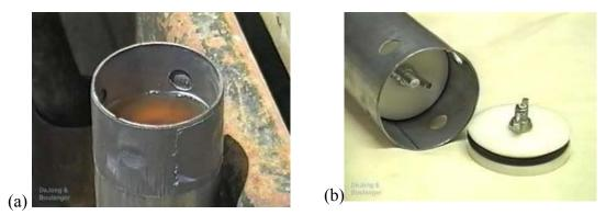
Figure 3-13. Shelby tube sealing methods, (a) Microcrystalline Wax, (b) O-Ring packer (FHWA, 2002b).
