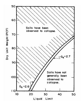
Figure 5-28. Chart for evaluation of collapsible soils (after Holtz and Hilf, 1961).
