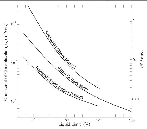
Figure 5-10. Approximate correlations between c<sub>v</sub> and LL (NAVFAC, 1986a).
