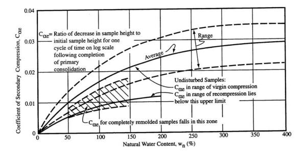
Figure 5-11. Correlation between C<sub>αe</sub> and natural water content (NAVFAC, 1986a).
