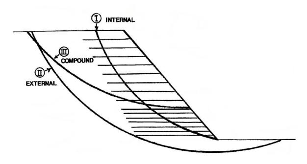
Figure 6-27. Failure modes for Reinforced Soil Slopes.
