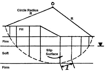
Figure 6-7. Geometry of Ordinary Method of Slices.
