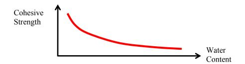
Figure 6-2. Effect of water content on cohesive strength of clay.
