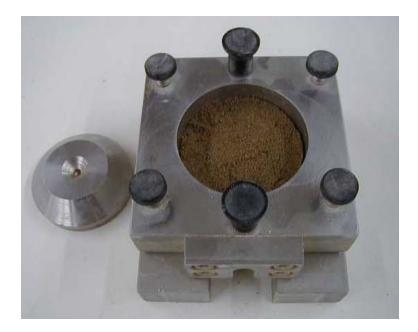
Figure 5-18. Direct shear testing box (Photograph courtesy of GeoComp Corporation).
