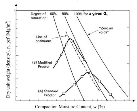
Figure 5-31. Compaction curves (after Holtz and Kovacs, 1981).
