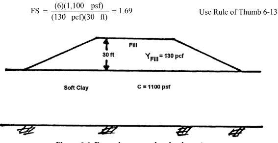
Figure 6-6. Example proposed embankment.
