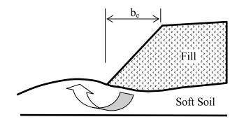
Figure 7-18. Schematic of lateral squeeze phenomenon.
