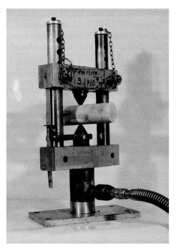
Figure 5-35. Point load strength test equipment (Wyllie, 1999).
