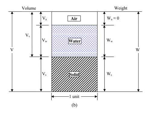
Figure 2-1. A unit of soil mass and its idealization.
