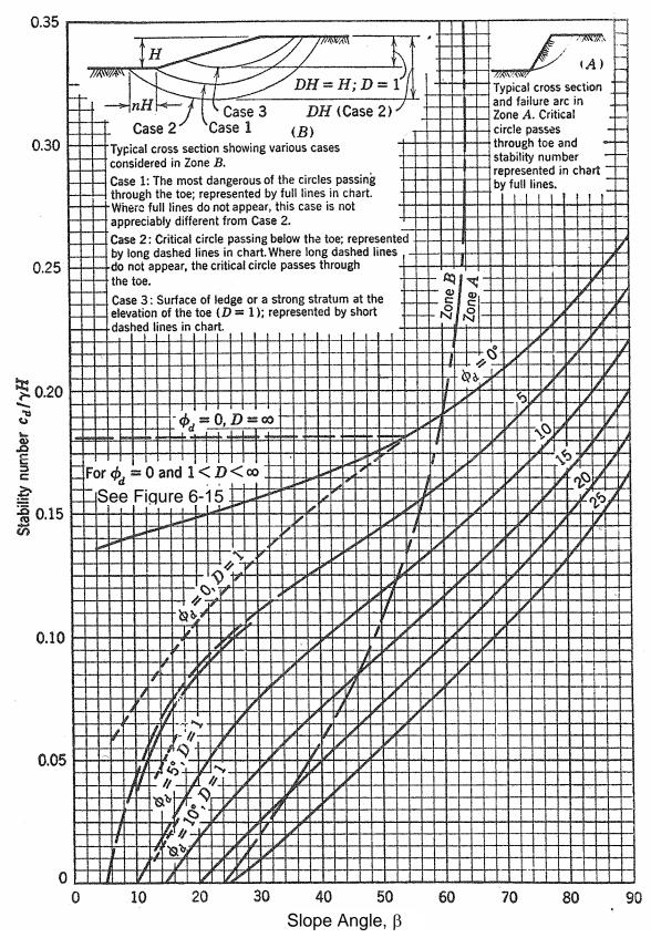
Figure 6-14. Taylor's chart for soils with friction angle (after Taylor, 1948).
