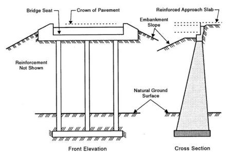
Typical Spill-Through Abutment
