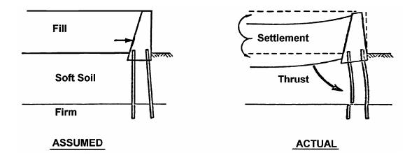
Figure 2-15. Schematic of effect of lateral stresses.
