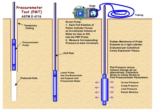
Figure 3-33. Pressuremeter test schematic (FHWA, 2002b).
