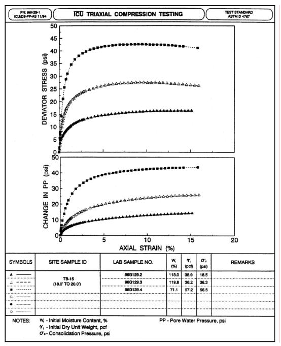
Figure 5-16. Typical stress-strain curves from CU test.
