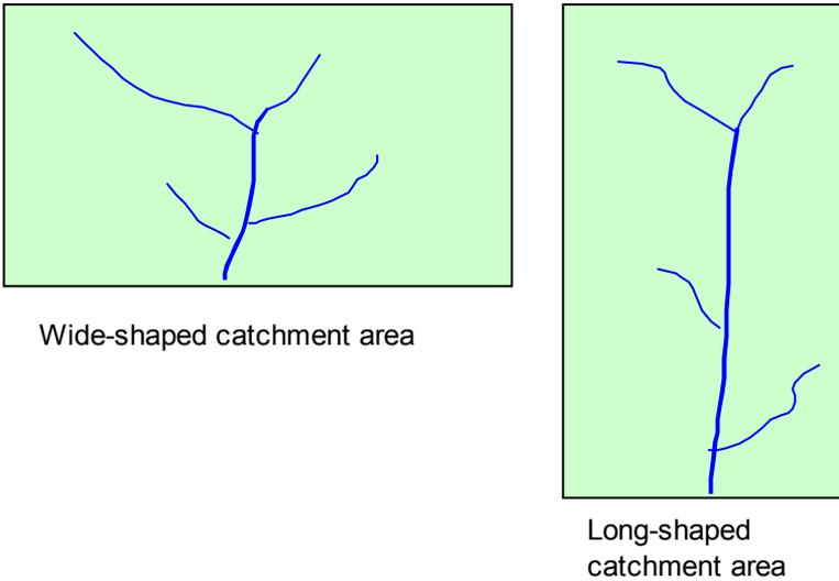
**Figure 3. Different shapes of catchment area.**
