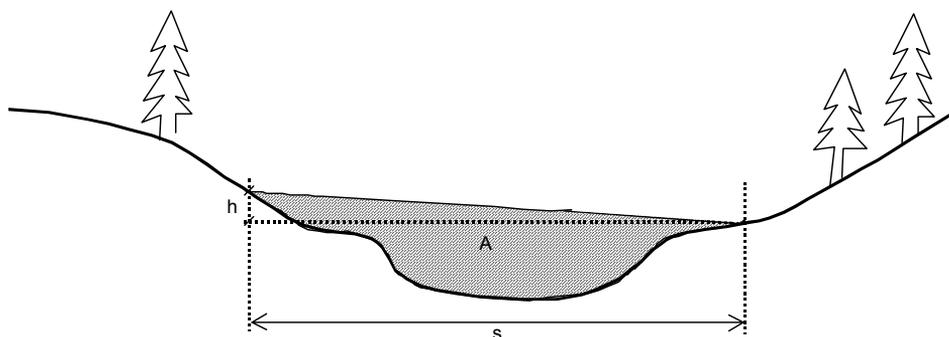
**Figure 6. Section for determination of flow velocity and flow.**
