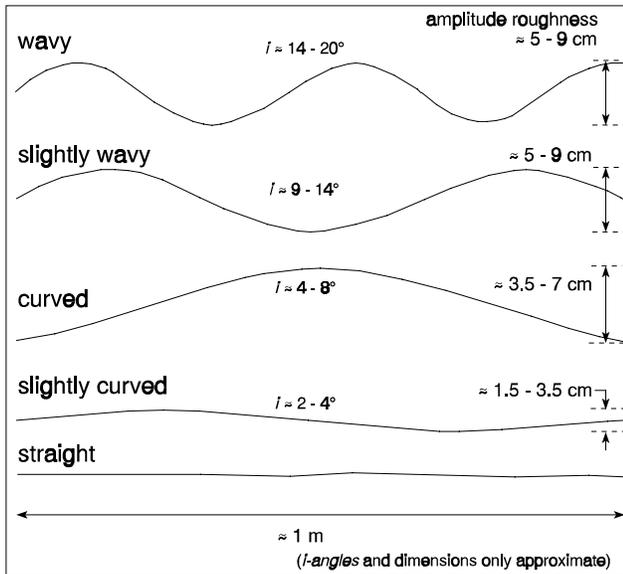
Fig. 3. Large scale roughness profiles.
