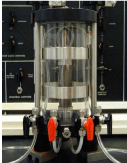
Figure 7-15. Permeameter Equipment: (a) Flexible-Walled Permeameter Cell; (b) Permeability Station with Automatic Volume Change Device (left) and Backpressure Panel Board (right side).
