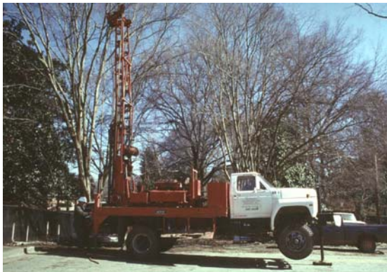
25. Views of Rotary Drill Rigs Mounted on Trucks for Soil & Rock Exploration.
