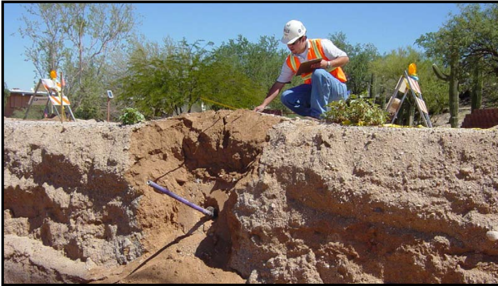
Figure 28. Passive failure where a hollow-core soil nail was tested close to the ground surface (see depression at the cut face and the profile at the ground surface above the soil nail).
