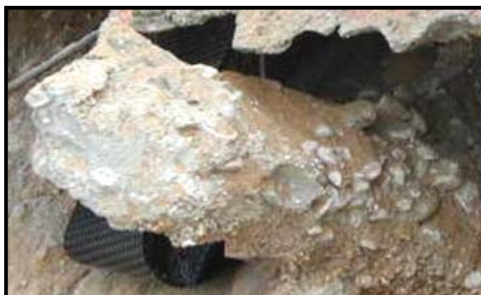
Figure 16. A 152 mm (~6-inch) diameter grout body generated by a 76 mm (~3-inch) cross-cut drill bit on an approximately 25 mm (~1-inch) outside diameter hollow-core soil nail.
