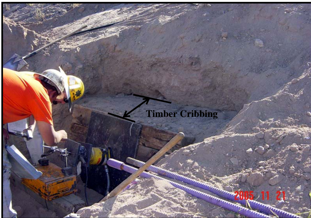
Figure 29. Timber cribbing reaction system embedded into slope to prevent passive failure during verification test of hollow-core soil nail.
