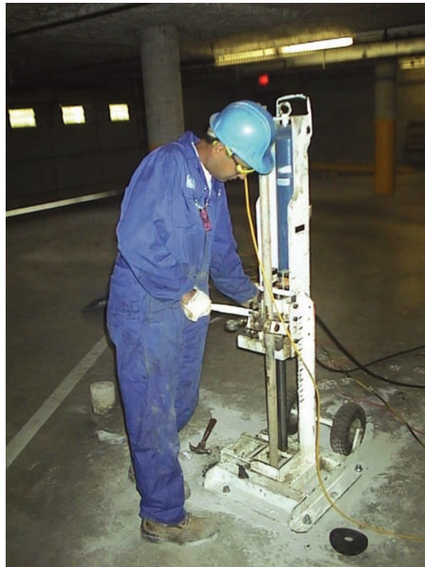
Figure 12 Ramset for CPT inside buildings or limited access
