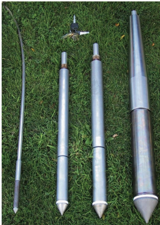
Figure 7 Range of CPT probes (from left: 2 cm 2 , 10 cm 2 , 15 cm 2 , 40 cm 2 )
