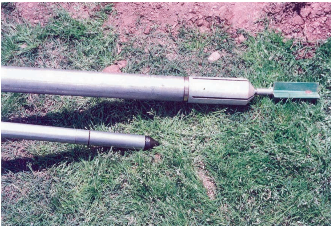
Figure 35 Typical field vane showing protective sheath for pushing in soft clays. A standard 10 cm 2 cone penetrometer is shown for scale.
