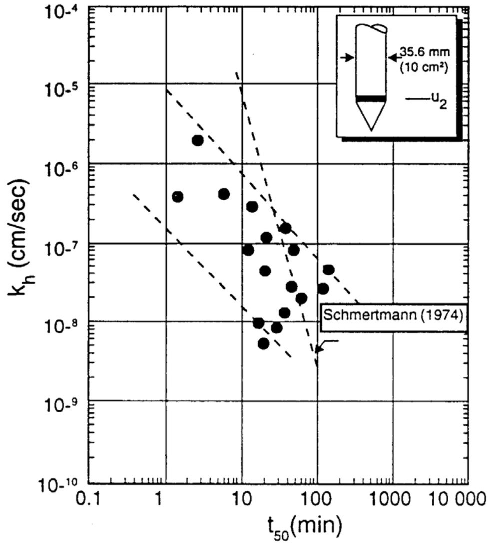
**Figure 25** Summary of data for estimating horizontal coefficient of permeability from dissipation tests (modified from Robertson et al., 1992).
