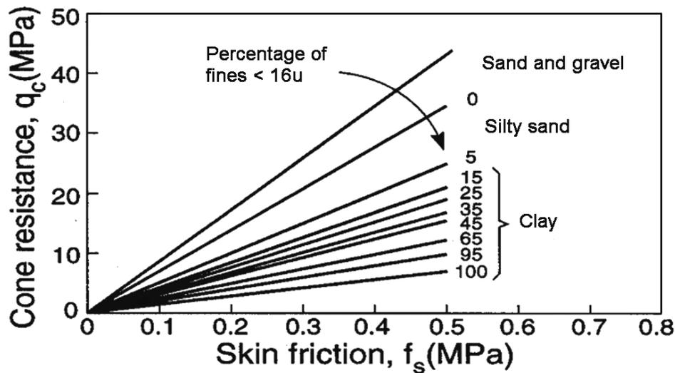
**Figure 6** First soil classification for Begemann mechanical cone
