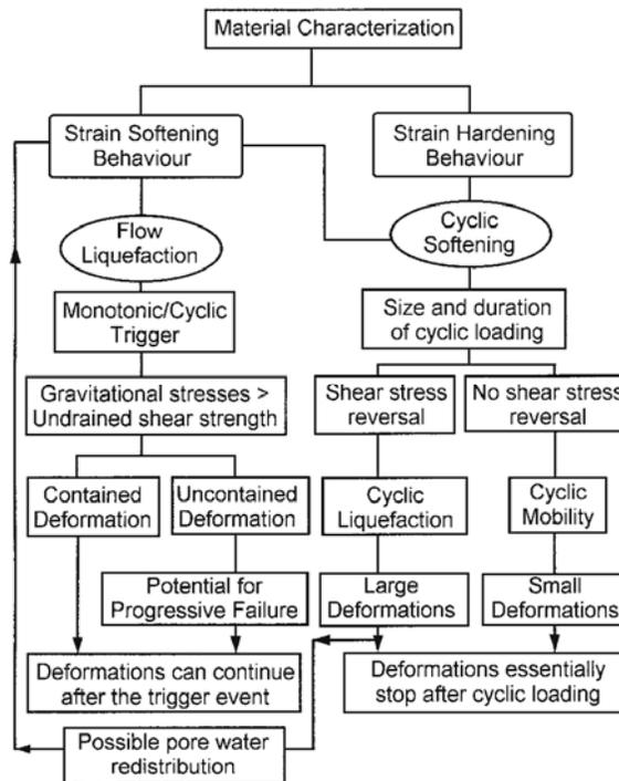
**Figure 35** Flow chart to evaluate liquefaction of soils.
