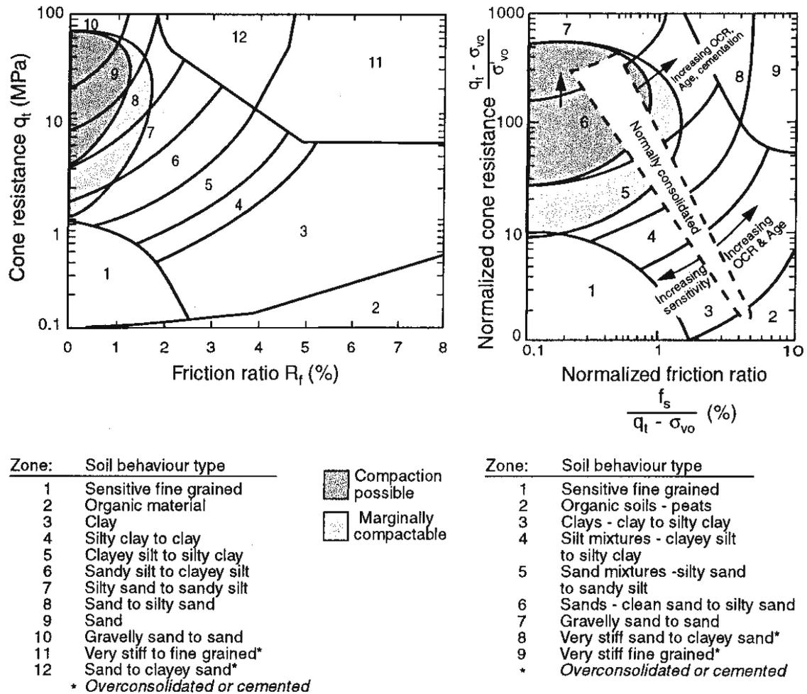
**Figure 41** Guidelines for soils suitable for vibrocompaction techniques.
