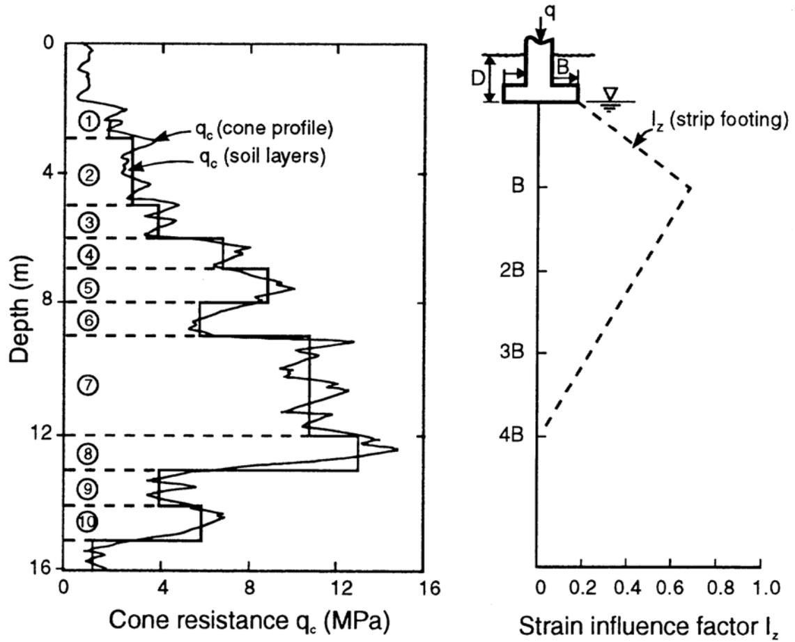
**Figure 31** Application of Schmertmann (1970) method for settlement of footings on sand
