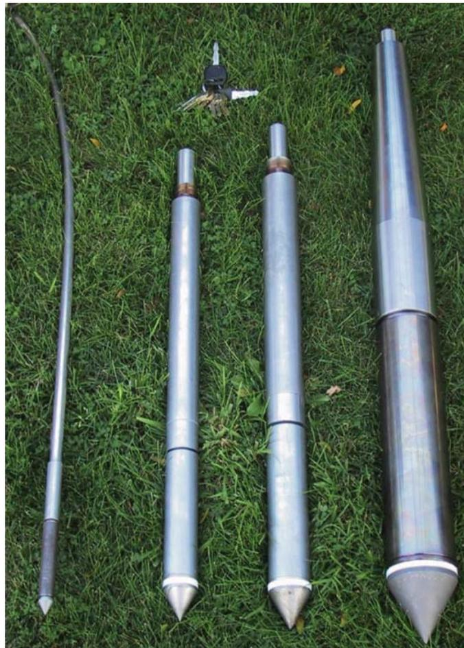
**Figure 7** Range of CPT probes (from left: 2 cm<sup>2</sup>, 10 cm<sup>2</sup>, 15 cm<sup>2</sup>, 40 cm<sup>2</sup>)
