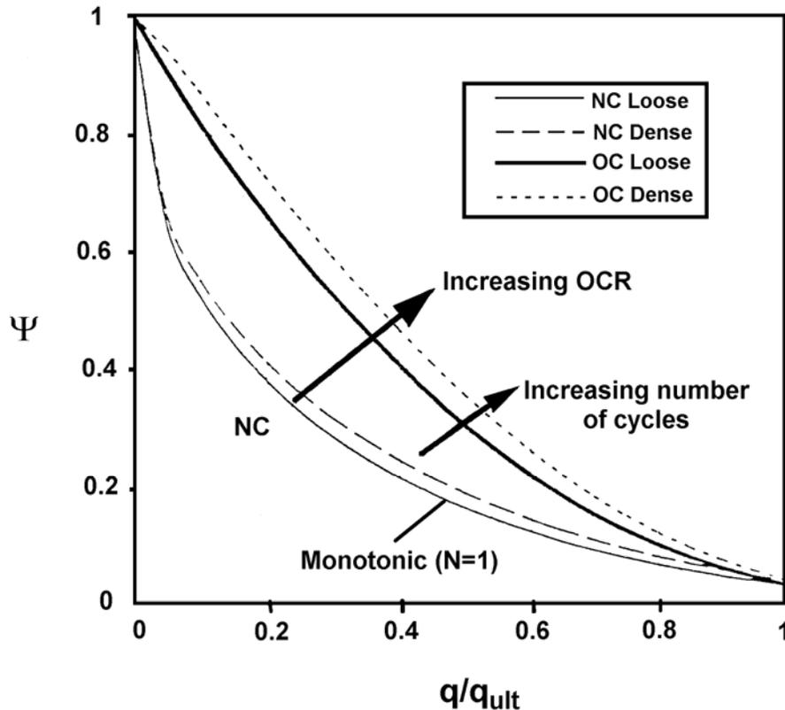
**Figure 32** Factor  $\Psi$  versus  $q/q_{ult}$  for sands with various densities and stress histories
