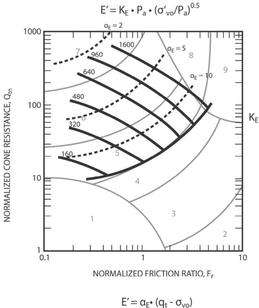
**Figure 22** Evaluation of drained Young's modulus from CPT for uncemented silica sands,  $E = \alpha_E (q_t - \sigma_{vo})$
