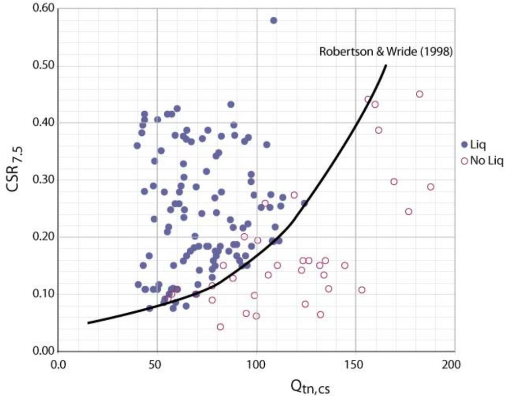
**Figure 36** Cyclic resistance ratio ( $CRR_{7.5}$ ) from CPT ( $Q_{tn,cs}$ )
