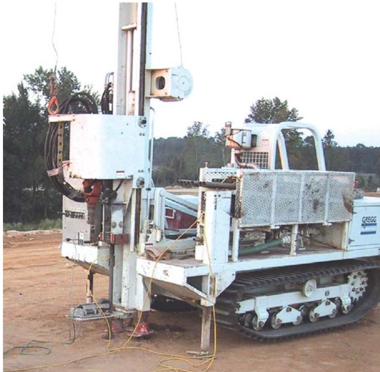
**Figure 11** Small anchored drill-rig unit
