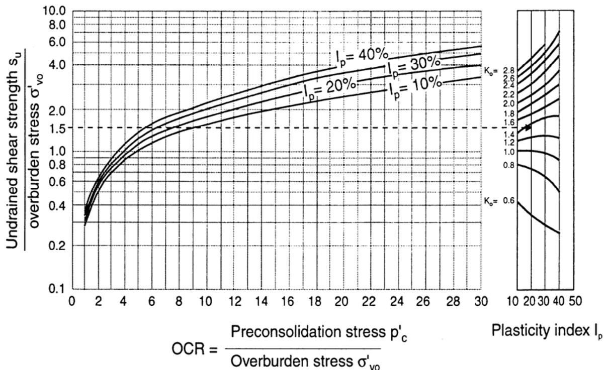
**Figure 20** OCR and  $K_o$  from  $s_u/\sigma'_{vo}$  and Plasticity Index,  $I_p$
