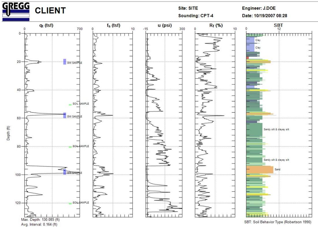
**Figure 18** Example CPTu profile with SBT
