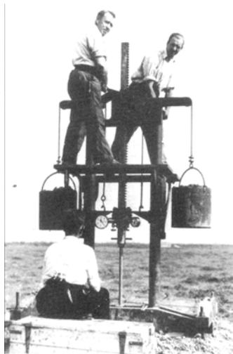
**Figure 3** Early Dutch mechanical cone (After Delft Geotechnics)
