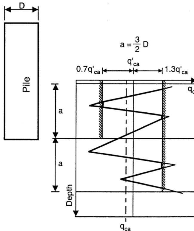
**Figure 34** Calculation of equivalent average cone resistance
