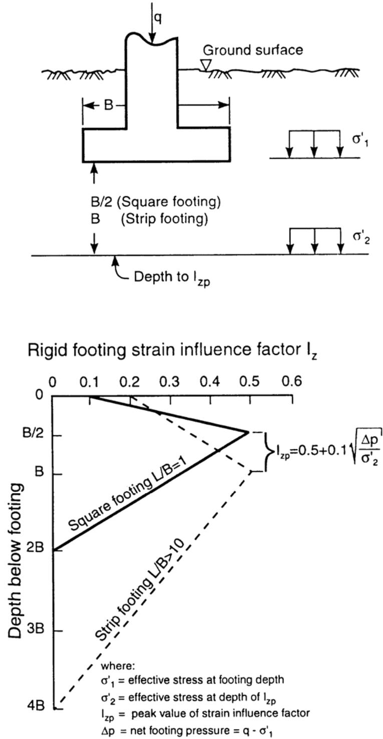
**Figure 29** Strain influence method for footings on sand (Schmertmann, 1970)
