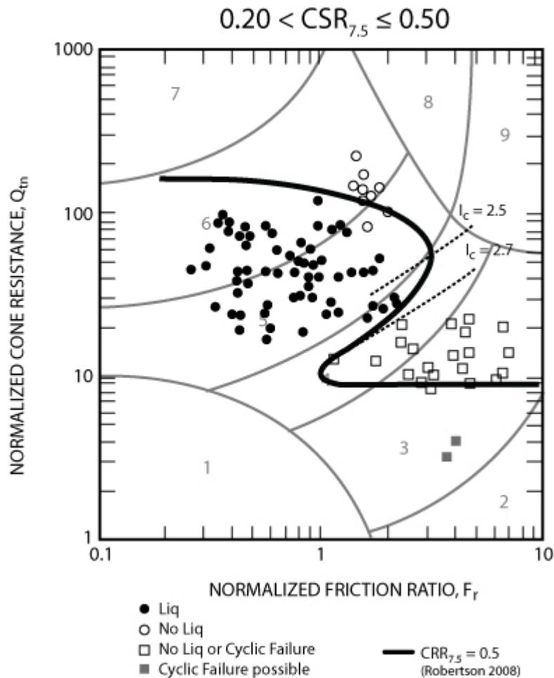
**Figure 39** Cyclic Resistance Ratio  $(CRR)_{M=7.5}$  using CPT
