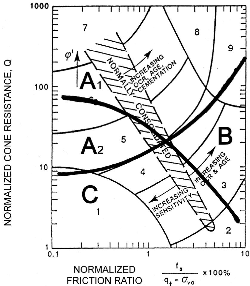
**Figure 40** Zones of potential liquefaction/softening based on the CPT
