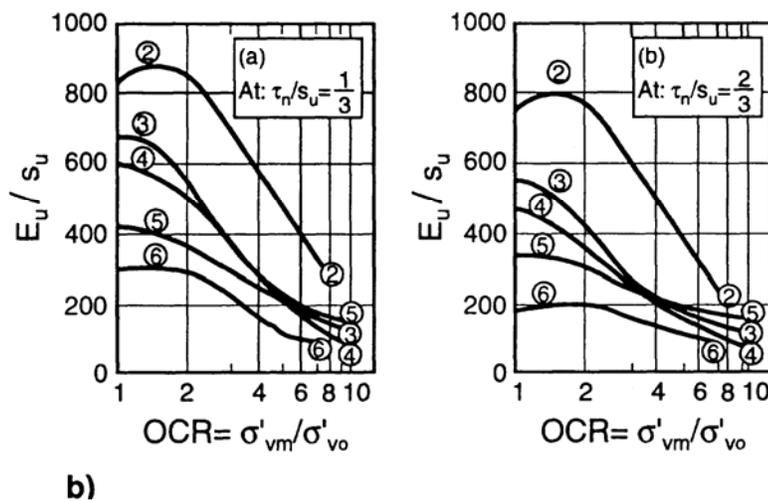
**Figure 33** Selection of soil stiffness ratio for clays
