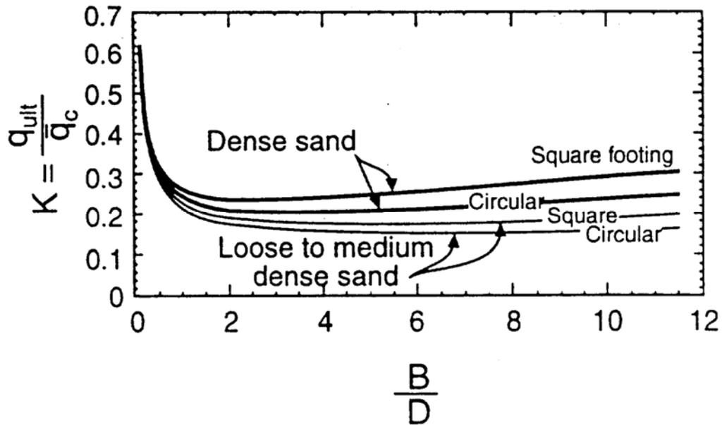
**Figure 27** Correlation between bearing capacity of footing on cohesionless soils and average cone resistance
