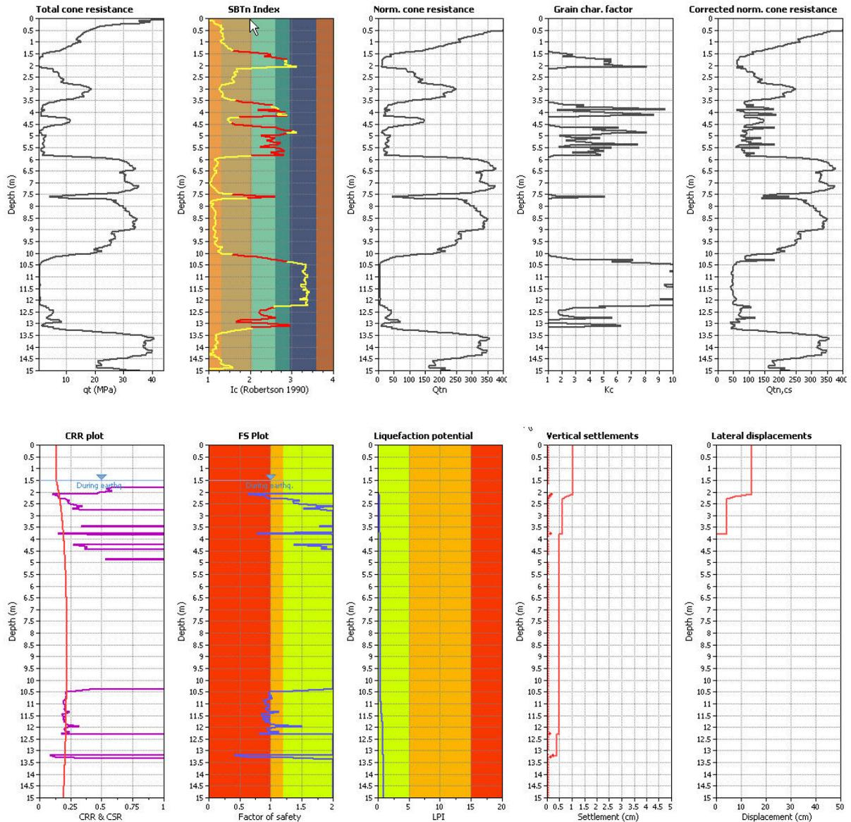
**Figure 38** Example of CPT-based approach to evaluate cyclic liquefaction/softening at Moss Landing Site showing (a) intermediate parameters (b) CRR, FS and post-earthquake deformations using ‘CLiq’ software (<http://www.geologismiki.gr/>)
