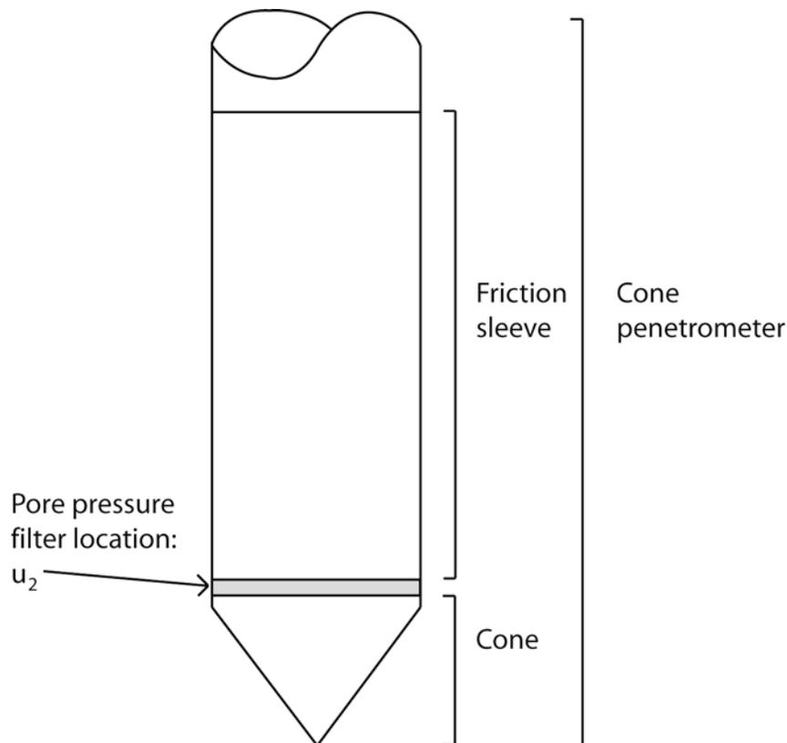
**Figure 1** Terminology for cone penetrometers
