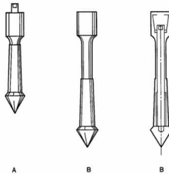
**Figure 4** Dutch mechanical cone penetrometer with conical mantle
