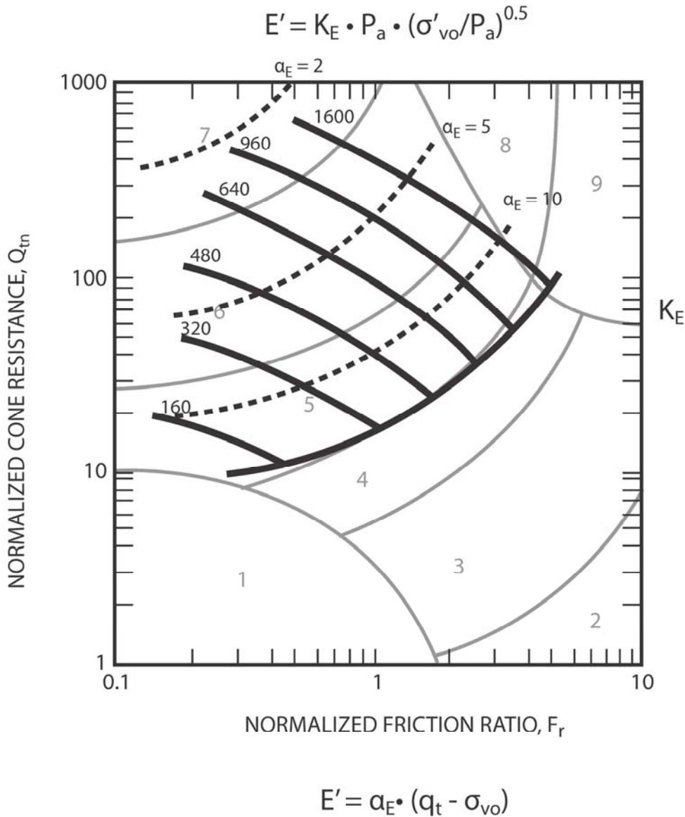
**Figure 30** Evaluation of drained Young's modulus from CPT for uncemented sandy soils,  $E = \alpha_E (q_t - \sigma_{vo})$
