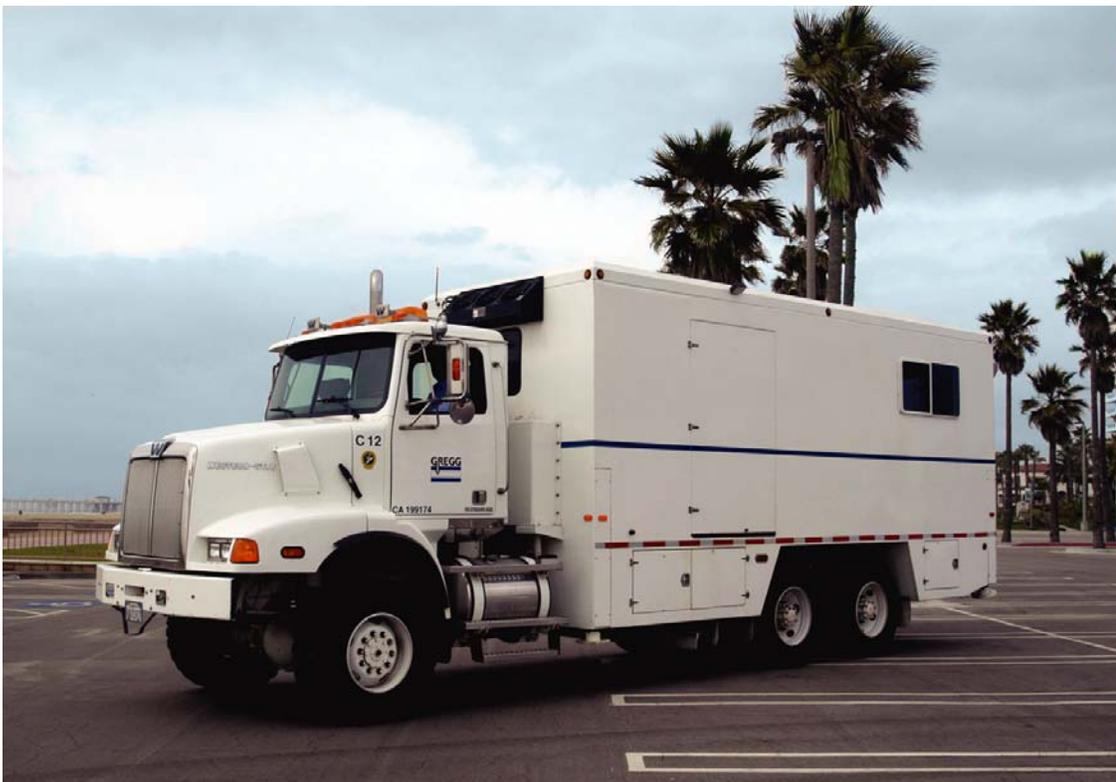
**Figure 9** Truck mounted 25 ton CPT unit
