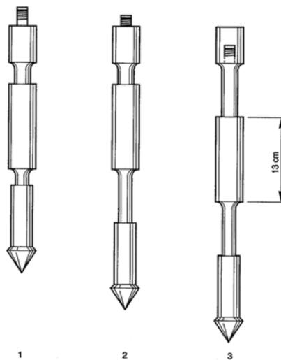
**Figure 5** Begemann type cone with friction sleeve
