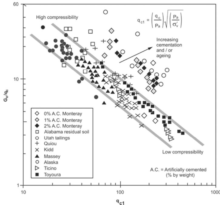
**Figure 24** Characterization of uncemented, unaged sands (after Eslaamizaad and Robertson, 1997)
