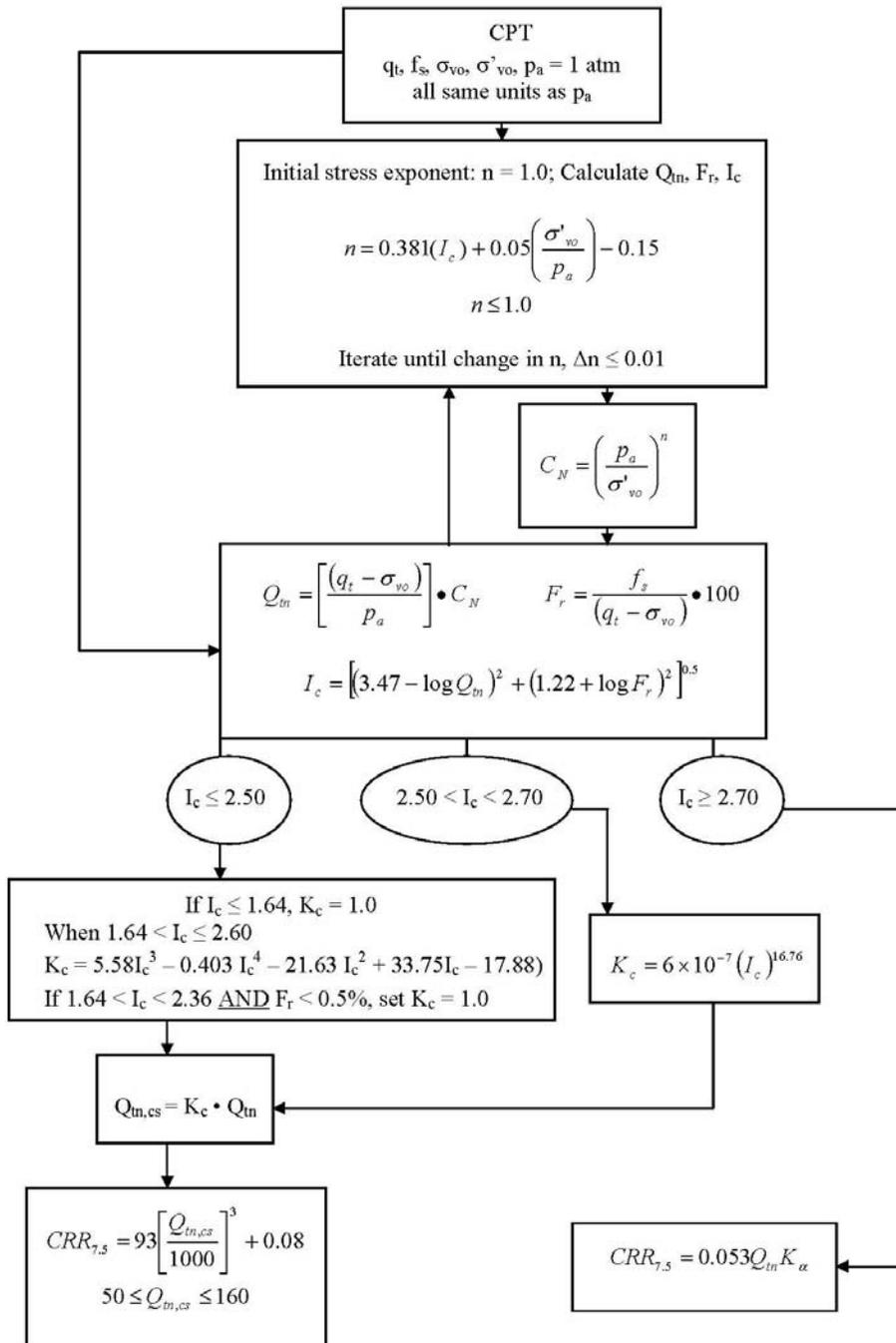
**Figure 37** Flow chart to evaluate cyclic resistance ratio ( $CRR_{7.5}$ ) from CPT (After Robertson, 2009)
