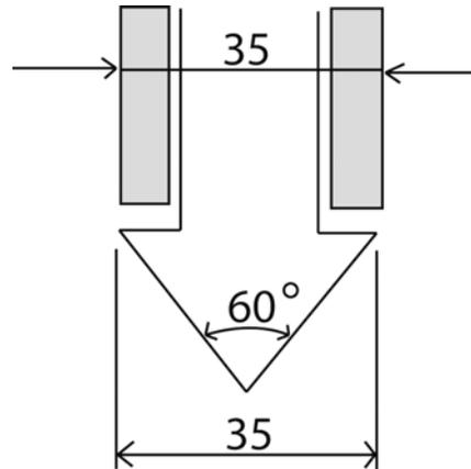
**Figure 2** Early Dutch mechanical cone (After Sanglerat, 1972)
