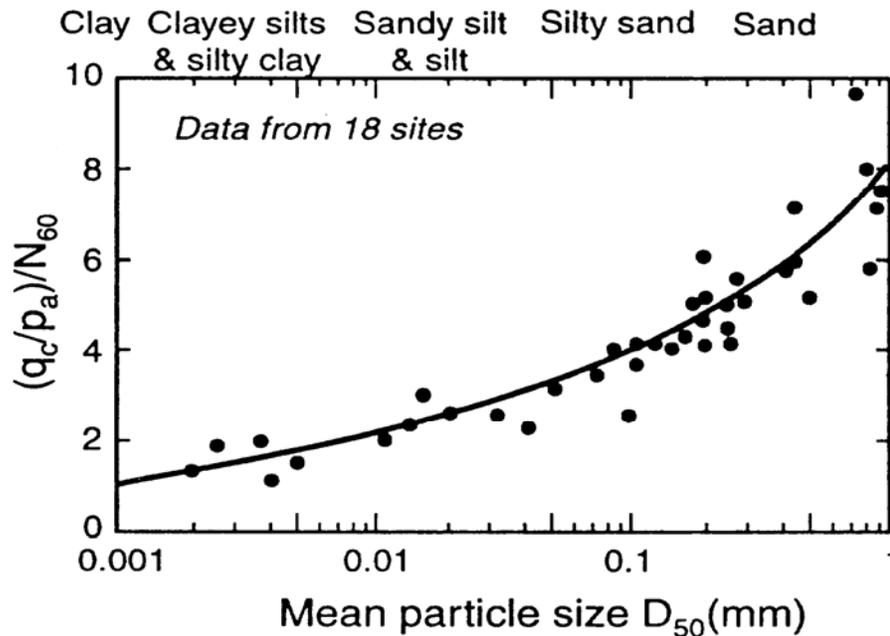
**Figure 19** CPT-SPT correlations with mean grain size
