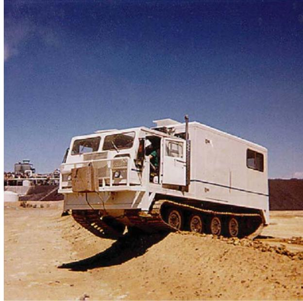
**Figure 10** Track mounted 20 ton CPT unit
