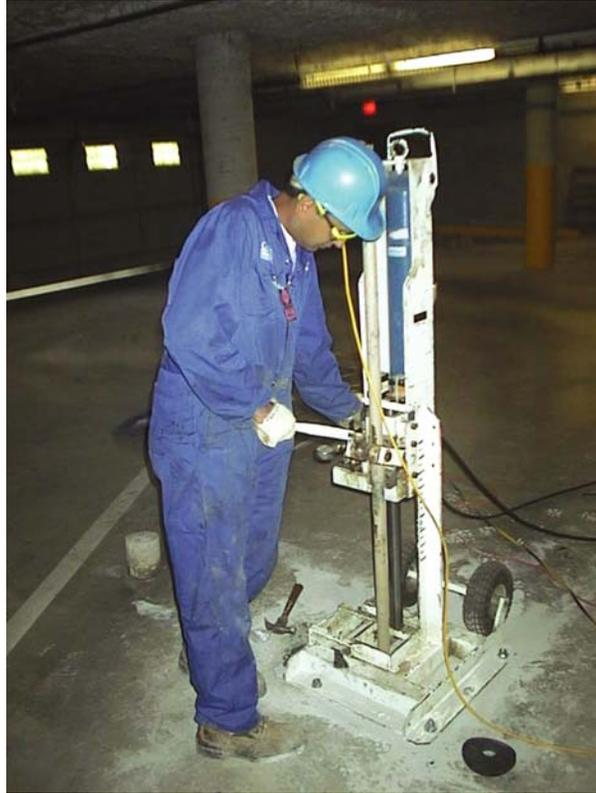
**Figure 12** Portable ramset for CPT inside buildings or limited access
