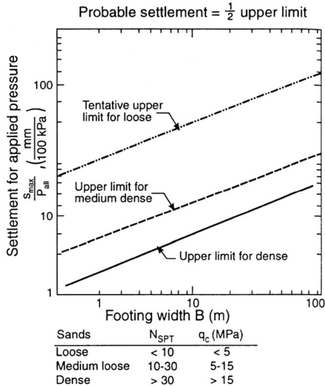
**Figure 28** Approximate range of settlement for footings in sand
