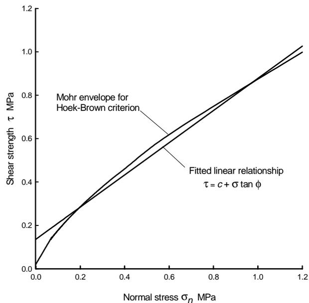
Figure 5. Mohr envelope for Hoek Brown criterion and fitted linear relationship for the normal stress range  $0 < \sigma_n < \sigma_v$  where  $\sigma_v =$  depth  $\times$  unit weight. As shown in the spreadsheet in Table 4, the friction angle  $\phi = 36.6^\circ$  and the cohesive strength  $c = 136$  kPa for  $\sigma_{ci} = 10$  MPa,  $m_i = 10$ ,  $GSI = 30$  and a depth below surface of 25 m.
