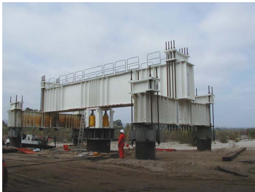
FIGURE 8-1 Static pile load test (five-pile array)
