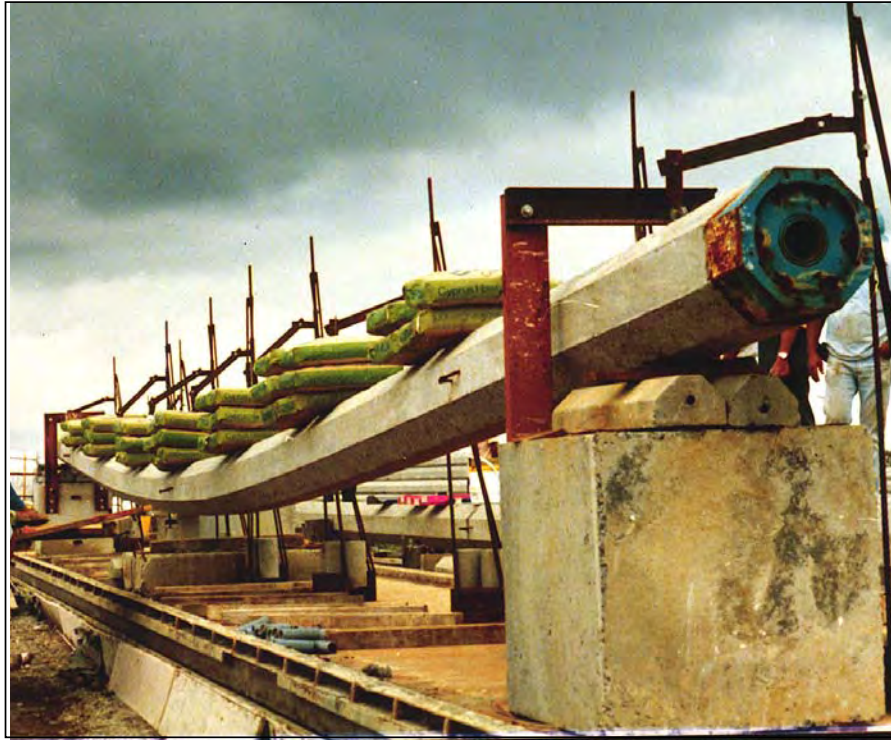
Fig. 7.31 Verifying the Principle of the curvature probe
