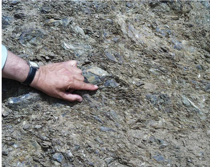
Figure 1: Appearance of sheared siltstone flysch in an outcrop
