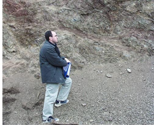
Figure 4 F. Tectonically deformed clayey shale or siltstone with broken sandstone
