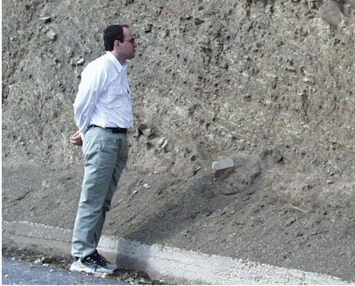
Figure 4 E. Weak siltstone or clayey shale with sandstone layers
