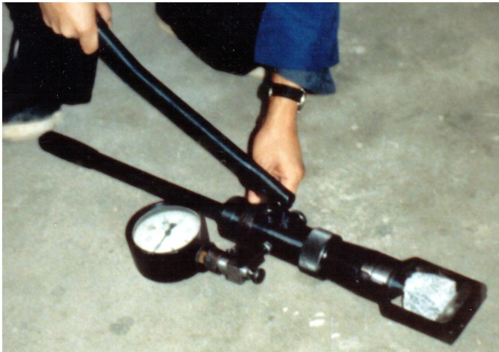
Figure 3: "Portable" point load test device for use in the field.
