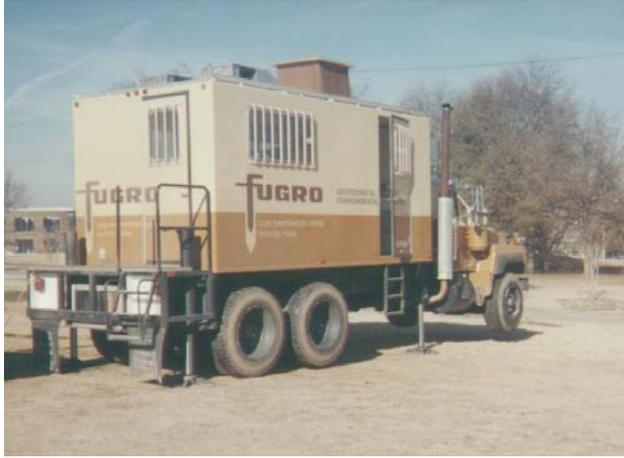
Figure 3. Closed-Cab Cone Truck in Georgia.
