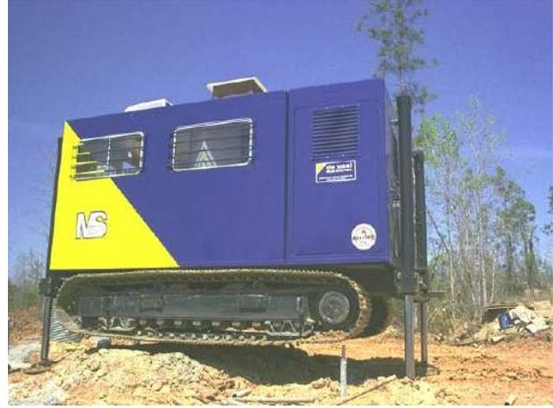
Figure 4. Track-Mounted Cone Rig in Alabama.
